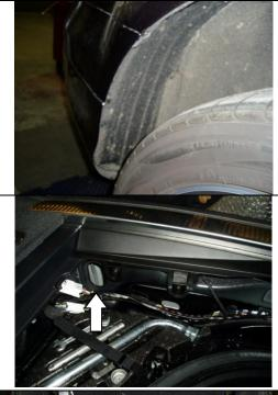
1. Remove torx screws around wheel arch and under the bumper profile.
