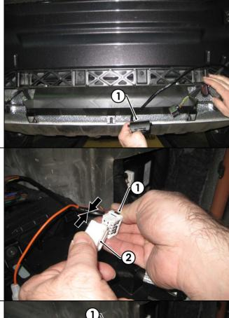
33. Connect the 8-way tail harness connector (1) to the trailer harness 8-way mating connector (2).
