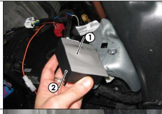
26. Mount the ECU (1) securely to the vehicle sheet metal as shown.
