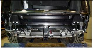
Remove 8 bolts holding impact beam.
