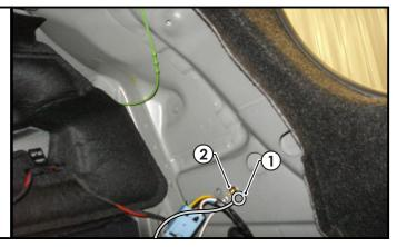
7. Connect the ORANGE 12v wire (1) to the positive side of the vehicle battery (2).
