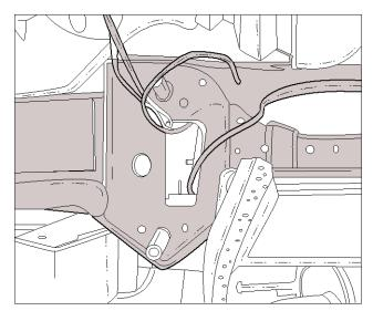
Cut of the bottom inside mounting face of the Impact Beam for the LH & RH side using the template provided on Page 8, rustproof the cuts and then remount the Impact Beam.
