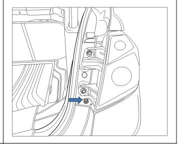
5. Remove 4x Nuts from the Impact Beam and remove Impact Beam.
