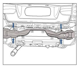
6. Mark and drill a \$12mm hole on the inside of the Chassis Rail for both the LH & RH side, position the hole 42mm from the bottom of the Chassis Rail and 56mm from the back face of the Chassis Rail (the face that the Impact Beam is bolted to).
