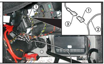
**6.** Connect the trailer patch ground ring terminal (1) to the vehicle grounding point (2).
