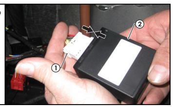
9. Apply double sided tape to the ECU (04838) (1) and secure it to the vehicle sheet metal in the area shown (2).
