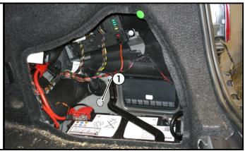
**4.** Following the table below, connect the ezy-taps (1) to the corresponding vehicle wires (2), then connect the trailer patch terminal (3) to the ezy-taps (1).
