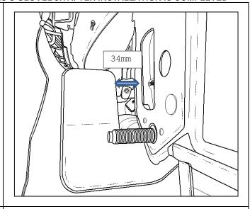
Thread the remaining wired Tapped Plates through the back face of the Chassis Rail and tighten all Bolts to the Torque Specifications provided and cut off the excess wire from the Tapped Plates.
