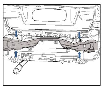
6. Mark and drill a ≥12mm hole on the inside of the Chassis Rail for both the LH & RH side, position the hole 42mm from the bottom of the Cassis Rail and 56mm from the back face of the Chassis Rail (the face that the Impact Beam is bolted to).
