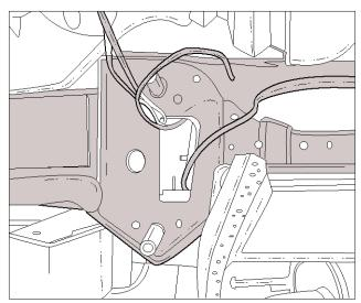
Cut of the bottom inside mounting face of the Impact Beam for the LH & RH side using the template provided, rustproof the cuts and then remount the Impact Beam.
