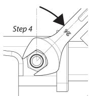
Fig 4. Tightening of Smart Pin Nut
