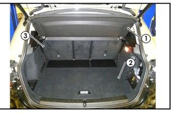
3. Remove the luggage compartment rear trim (1) by removing four clips (2).
