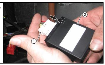
9. Apply double sided tape to the ECU (P/No: 04838) (1) and secure it to the vehicle sheet metal in the area shown (2). Note: Ensure to mount the ECU with the connector facing downwards.
