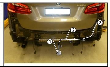
**19.** Connect the tail harness 8-way connector (1) to the trailer wiring harness mating 8-way connector (2).
