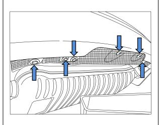
6. Where installed, remove 4x Heat shield fasteners and 2x Screws; remove lower section of heat shield, ensuring heat shield is lifted over locators.
