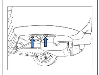
Remove 6x (8x where lower Heat Shield is install) Screws from underside of bumper, at rear end of vehicle.
