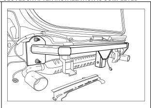
Where installed, identify centreline of lower heat shield removed in step 6. Create a cutout as per diagram. Cover cut edge using pinch weld provided.
