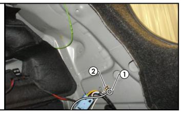
7. Connect the ORANGE 12v wire (1) to the positive side of the vehicle battery (2).
