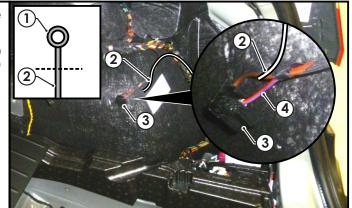
**13.** Secure the trailer patch ground ring terminal (1) to the vehicle grounding point (2) using the existing vehicle fastener (3).
