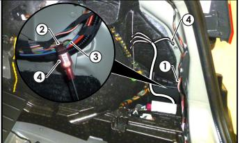
Gain access to the vehicle harness wires by un-taping the vehicle harness in the area roughly highlighted (1).
