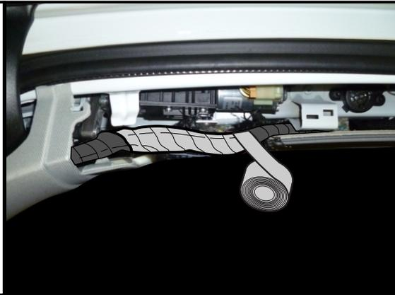
17. Connect the trailer patch connector (1) to the ECU (2). Remove the backing from the back of the ECU and mount the ECU (2) onto the sheet metal area (3). Ensure ECU is mounted with the connector pointing downwards.
