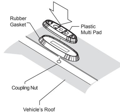
**STEP 4: Fitting the Cross Bars to the Vehicle**
