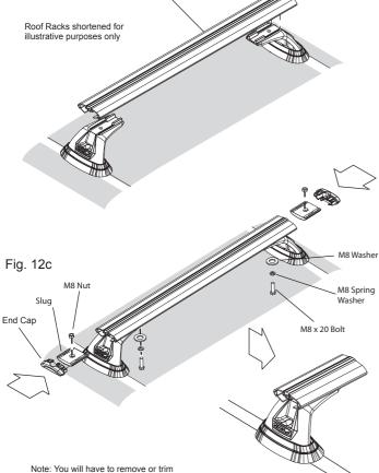
Fitting the Cross Bars to the Vehicle
