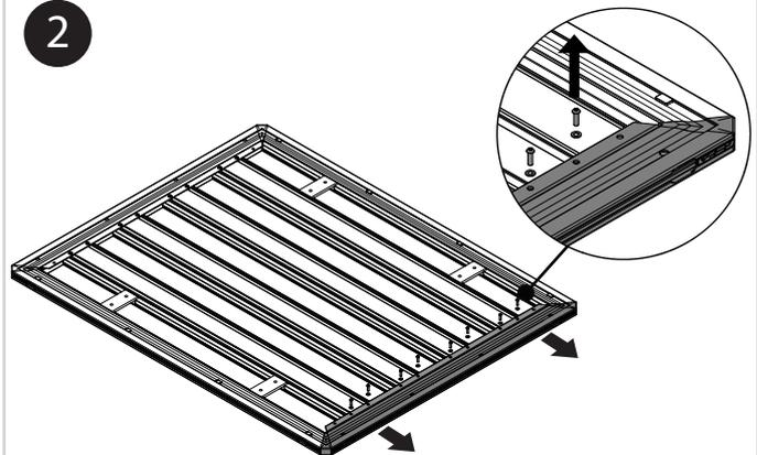
Place tray upside down. Remove fasteners on one side and remove the end plank.
