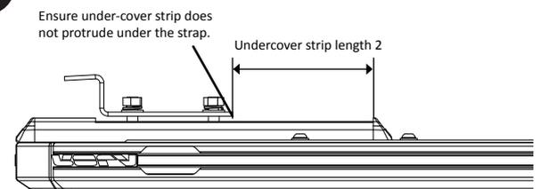
While the tray is upside down, cut and insert under-cover strip lengths for the inner side of each Low Mount.
