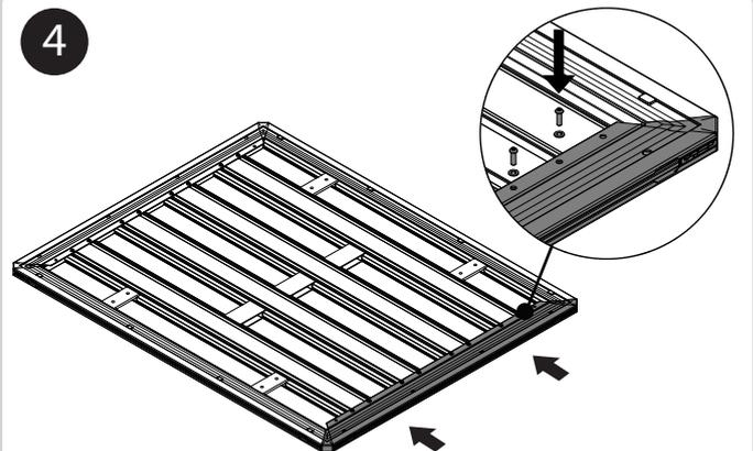
Re-install the end plank and fasteners.
