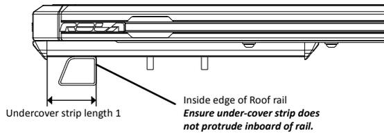
Cut the under-cover strip to the required lengths for each Low Mount.
