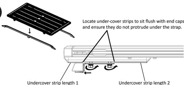
Place tray on roof rails and slide the rail straps in place under the vehicle roof rail.
