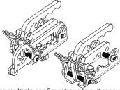
The RCHLJ has multiple configurations to suit many jack types. One unit is equiped with a support anc clip to retain your jack handle. Where possible, this unit should be positioned toward the top end of the jack. The RCHLJ comes pre-assembled but must be tightened before use. Before tightening check that the current configuration suits your jack. If it does not, change the configuration to suit your particular jack. (Refer Step 2) Once configuration is set tighten all fasteners.
