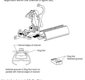
Tighten bolt and re-install Buffer Strip
