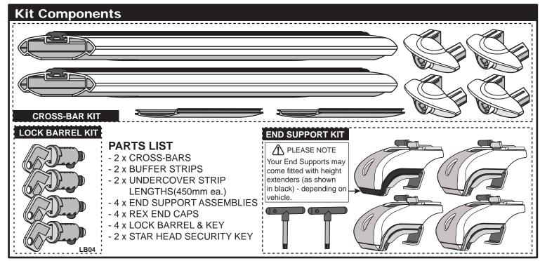
TOOLS REQUIRED: Cutting Blade, Lead Pencil, Steel Rule, Measuring Tape - Please read instructions thoroughly before commencing installation.
