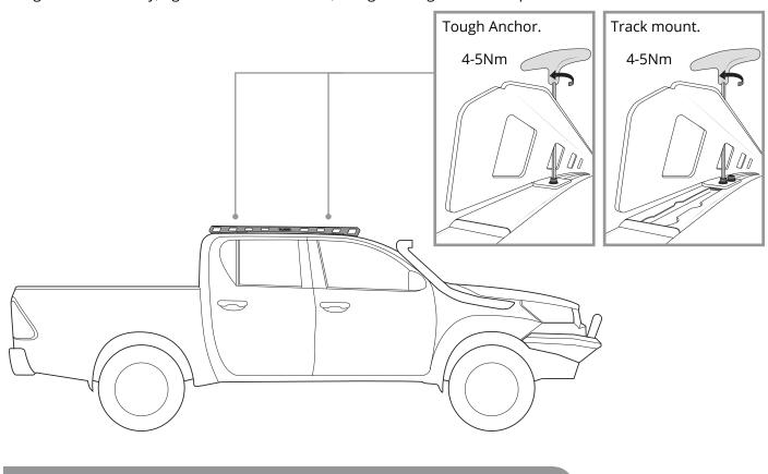
Install the stud plates as shown.
