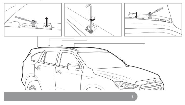
Remove the rails from the roof of the vehicle.
