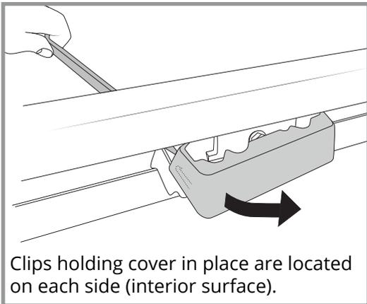
Clips holding cover in place are located on each side (interior surface).
