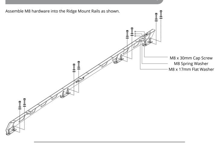
Install the Ridge Mount hardware as shown below. Tighten with a 13mm spanner.
