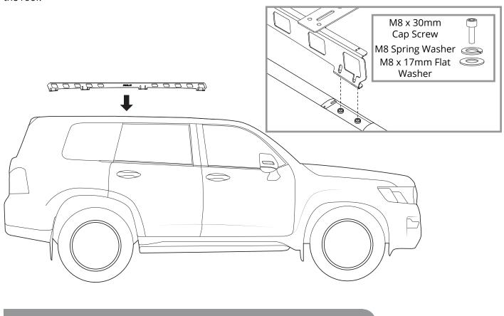
Tighten the M8 hardware with a 6mm allen key to 4-5Nm. Note: Access hardware through cutouts on side or holes located on top of the rail.
