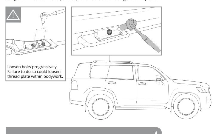
Carefully remove the factory rails. Clean the roof of the vehicle thoroughly.
