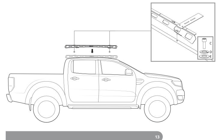
Tighten the M6 hardware with a 5mm allen key to 4-5Nm. Note: Access hardware through cutouts on side of the rail.
