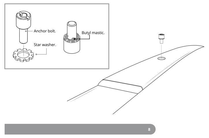
Hold the anchor bolt in place with a wide flat head screwdriver and secure with an M6 nyloc nut, using a 10mm socket.
