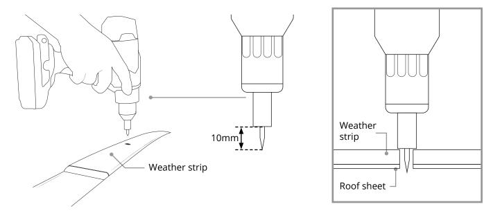
Use a 11mm drill bit and open up the hole in the weather strip made previously. Do not drill through the sheet metal. Using a drill stop and incrementally increasing depth will ensure roof sheet will be protected.
