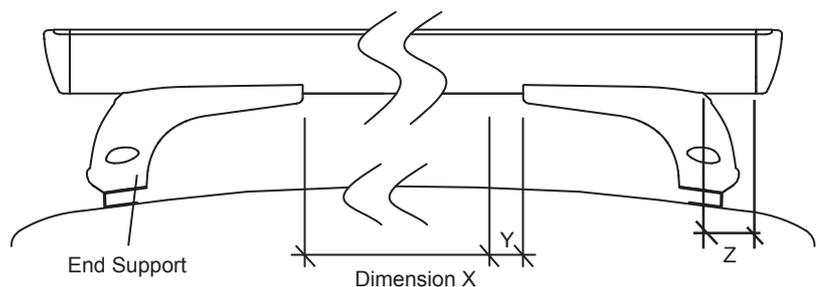
(Measured between End Supports for H/D type bar (Dim. X) or from End Support to edge of cutout for Sports bar (Y))
