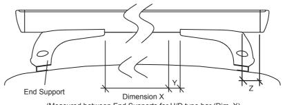
(Measured between End Supports for H/D type bar (Dim. X) Fig. 5 or from End Support to edge of cutout for Sports bar (Y))
